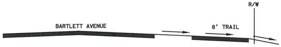
RURAL SECTION - REVERSED TRAIL SLOPE
