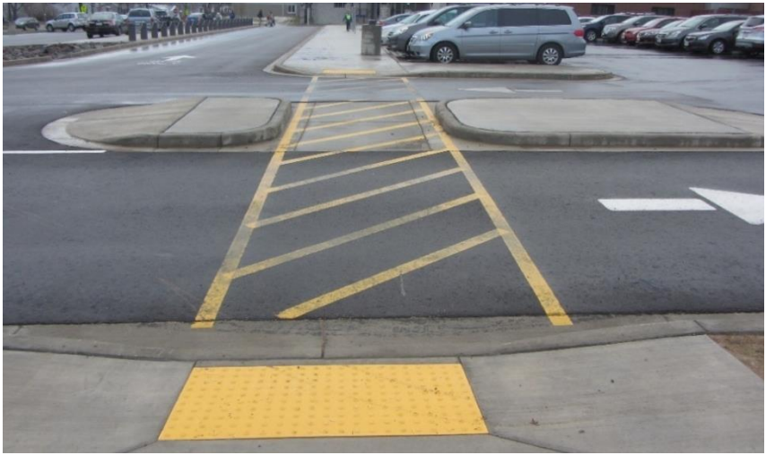
This on-site crossing of a parking lot entry of the Altoona School District Campus utilizes a refuge island and patterned crosswalk.
